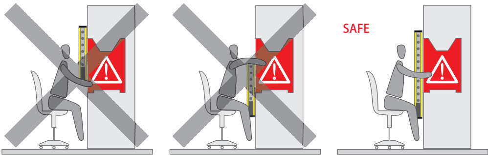
FIG. 4: POSITIONING THE LIGHT CURTAIN
