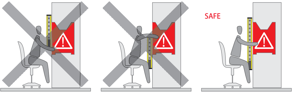
FIG. 9: POSITIONING THE LIGHT CURTAIN
