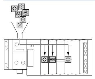
The valves of the Motion Terminal VTEM comprise four 2/2-way valves with piezo pilot control connected to form a full bridge, monitored by sensors.
