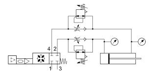
A desired setpoint value can be specified for ducts 2 and 4 independently of each other.
