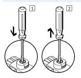
1 Press in the stem of the MO with a pin or screwdriver. Pilot valve switches and actuates the main valve.
