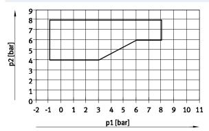
For polymer poppet valve in width 10 mm with code: MU, NU, KU, HU
