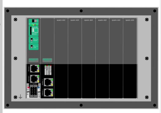
Figure above: View to rear side and connections sides of PC717T-PNC
