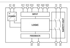
Fig. 1 Block diagram ESM-2H2..
