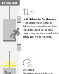
Elimination of the mechanical overspeed governor: In case of overspeed the safety circuit will be open respectively the electromechanical safety gear will be triggered by the Kübler Safe System.
