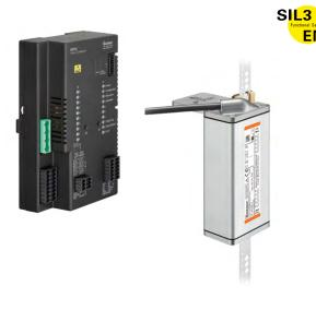
To trigger electromechanical safety gears, the SIL3-certified sensor Ants LES03 can be combined with the SIL3-certified Safety Gear Trigger SGT02. This means that classic mechanical solutions with all the relevant components can be replaced. This reduces both the complexity in the installation process and the number of components in the safety circuit of the elevator system.
