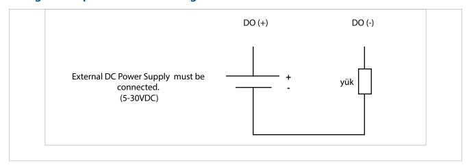
Fig. 2-2 Digital Output Connection Diagram ( POWYS 10xx )
