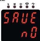
Press the right button so that "NO" sign starts blinking. Then, press the left button to exit the menu without saving the changes made.
