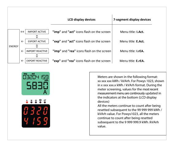
Fig. 3-3 Example of Import Active Energy Meter Display
