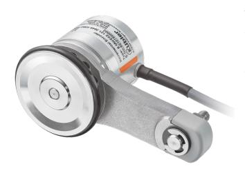
The MWE02 measuring wheel system is the ideal solution for reliable speed, position and distance measurement in applications with linear movements. These are recorded rotationally via the measuring wheel with attached encoder and converted into measurement data.
