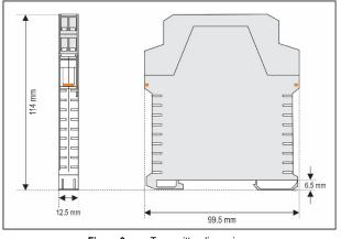
Figure 9 – Transmitter dimensions
