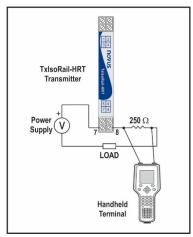
Figure 7 – Handheld terminal connection
