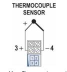
Figure 14 – Thermocouple connections
