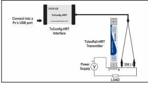
Figure 1 – TxConfig-HRT interface connection to the TxIsoRail-HRT
