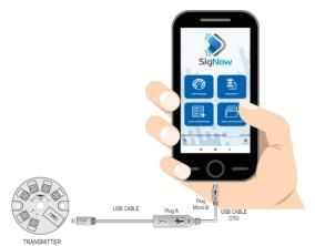
Figure 13 - On the Go connection cable
