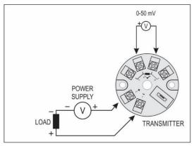
Figure 7 - Transmitter electrical connections (0-50 mV)
