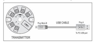
Figure 8 - USB cable connection
