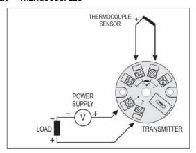
Figure 6 - Transmitter electrical connections (Thermocouple)
