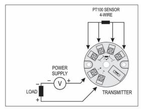
Figure 4 - Transmitter electrical connections (Pt100 4-wire)
