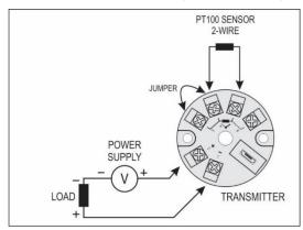
Figure 2 – Transmitter electrical connections (Pt100 2-wire)
