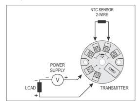
Figure 5 - Transmitter electrical connections (NTC 2-wire)
