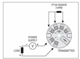
Figure 3 – Transmitter electrical connections (Pt100 3-wire)
