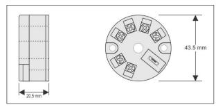
Figure 1 - Transmitter dimensions
