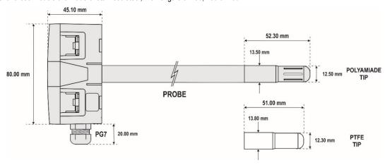
Figure 17 – DM model dimensions
