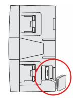
Figure 22 – USB cable connection
