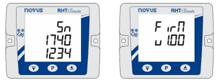
Figure 26 – Serial number and firmware version information
