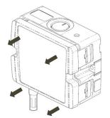
Figure 19 - Removing the front cover of the transmitter
