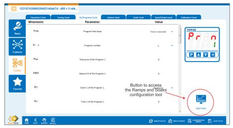
Figure 24 Button for the Ramps and Soaks tool
