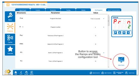
Figure 16 Ramps and Soaks Tool Button
