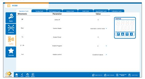
Figure 20 Cycles of a standard controller
