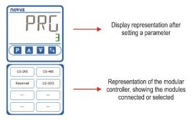
Figure 22 Dynamic display of the modular controller
