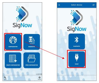
**Figure 1** – Establishing a TCP/IP connection
