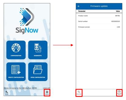
Figure 23 – Upgrading firmware via app
