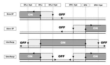
Figure 7 - Conditions of activation and deactivation of the different alarm modes
