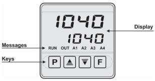
Figure 2 - Front panel identification
