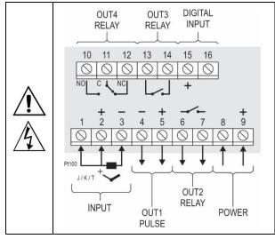
Figure 1 - Electrical connections
