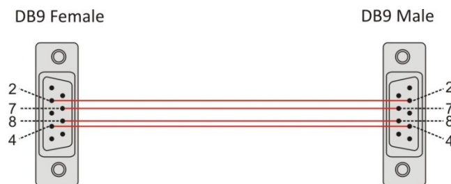
Figure 112 – Building an extension cable
