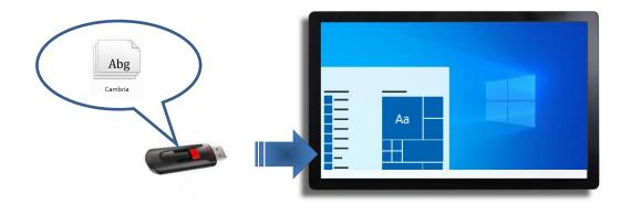
Occasionally the font displayed in the SCADA program is not the same as that in the editor. This might be resulted from missing fonts in the SCADA program, which is run on a different PC rather than the one for project editing.
