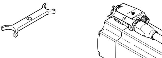
The spanner is included in the scope of delivery of the motor cable.
