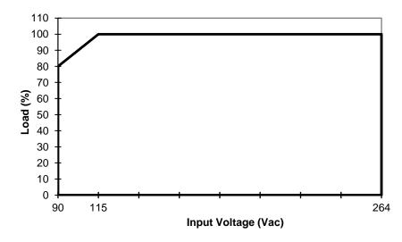
No output power de-rating for the input voltage 115 Vac to 264 Vac
