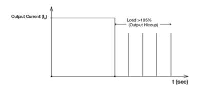
Additionally, if the Io is < 105% but > 100% for a prolong period of time (depending on the load), the Over Temperature Protection (OTP) will be activated due to high temperature on critical components. The power supply will then go into "Hiccup mode" until power supply cool down.
