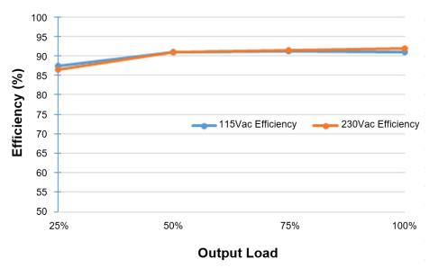
Fig. 1 Efficiency versus Output load
