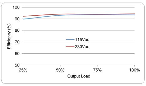
Fig. 1 Efficiency versus output load
