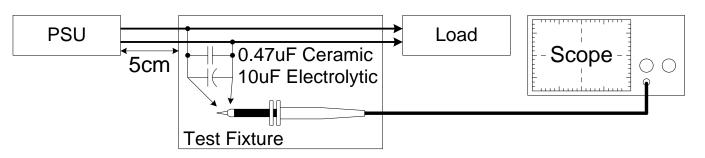
Fig. 3 Ripple & Noise measurement circuit
