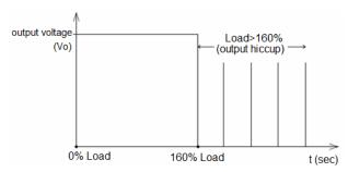
Additionally, if the 24 Volts' lout is >100%; but <160% for a prolonged period of time (depending on the load), the Over Temperature Protection (OTP) will be activated due to high temperature on critical components. The power supply will then go into latch mode.
