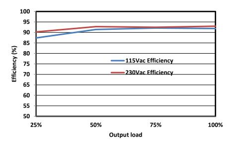
Fig. 1 Efficiency versus output load
