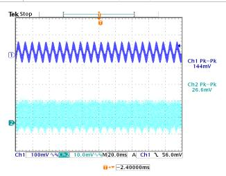
(a) 115 V (measured value=138.0 mV for 24 V and 35.0 mV for 5 V)
