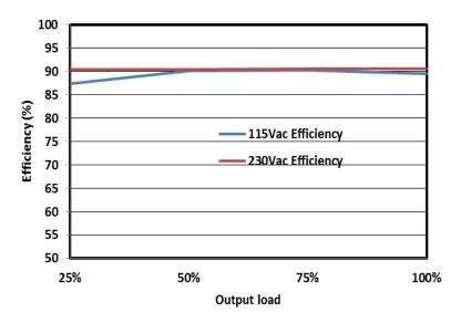
Fig. 1 Efficiency versus output load
