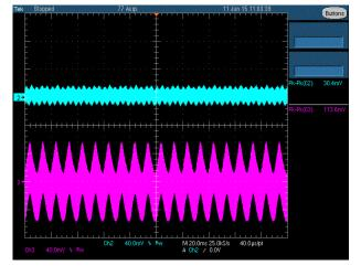
(a) 115 V (measured value=112.0 mV for 12 V and 28.8 mV for 5 V)
