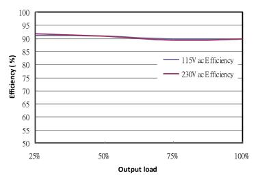
Fig. 1 Efficiency versus output load
