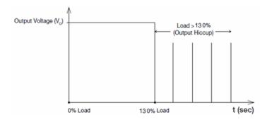
Additionally, if the lo is <130% but >110% for a prolong period of time (depending on the load), the Over Temperature Protection (OTP) will be activated due to high temperature on critical components. The power supply will then go into hiccup mode until the fault is removed; and, the input voltage is removed, then reapplied.
