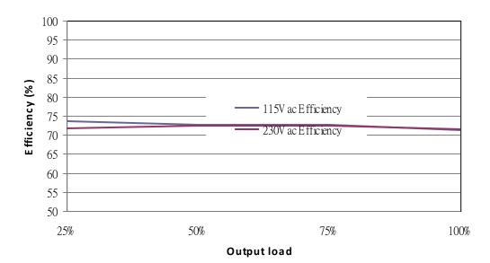
Fig.1 Efficiency versus output load
