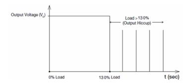
Additionally, if the I<sub>o</sub> is <130% but >110% for a prolong period of time (depending on the load), the Over Temperature Protection (OTP) will be activated due to high temperature on critical components. The power supply will then go into hiccup mode until the fault is removed; and, the input voltage is removed, then reapplied.
