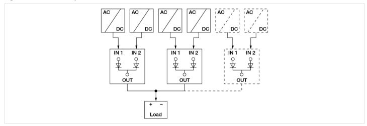
Connecting only one PSU to one DRR module to reduce the stress of the diodes and hence increase the reliability.
