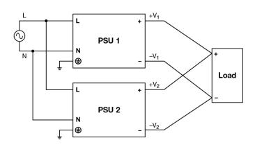
Fig. 4 Parallel Operation Connection Diagram
