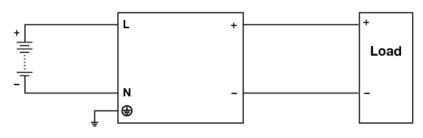
Fig. 6 DC Input Operation Connection Diagram
