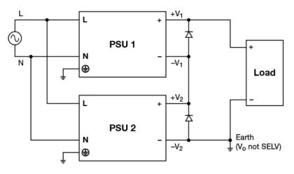
Fig. 5 Series Operation Connection Diagram
