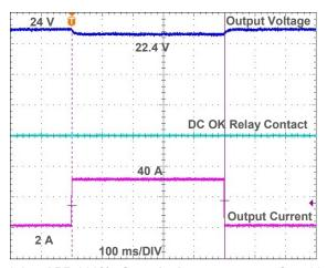
Fig. 8.2 APB 200% of nominal output current for 500 ms
