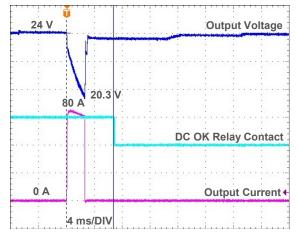
Fig. 8.3 APB 400% of nominal output current for 2 ms
