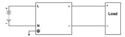
Fig. 4 DC Input Operation Connection Diagram
