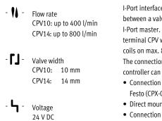
I-Port interface for communication between a valve terminal CPV and an I-Port master. It activates a valve terminal CPV with up to 16 solenoid coils on max. 8 valve positions. The connection to a higher-order controller can be achieved by:
