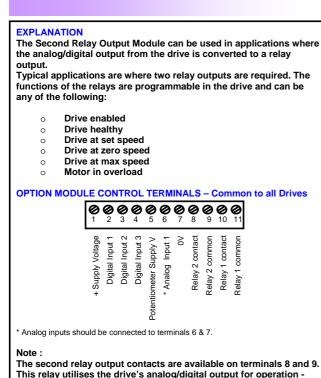
This relay utilises the drive's analog/digital output for operation therefore the analog output is not available when this module is fitted.
