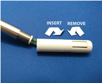
Fig. 3 – Installation of the tip in the device
