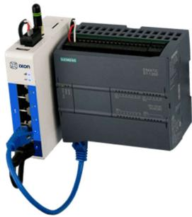
Each IXrouter has four ethernet ports for connecting machines (PLCs and machine networks) and robots, and one WAN port to connect it to the internet. There are multiple versions of the IXrouter supporting additional ways to get internet access:
